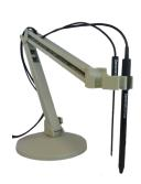
The probe stand can fit probes and includes 2 adapter rings for mounting probes with various shapes and dimensions.
